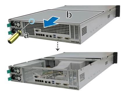
**Note:** When you remove the rear top cover, sensitive internal components are exposed. Avoid touching anything other than the memory assembly when removing or adding memory.
