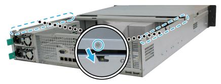
**b** Put back and fasten the screw you removed in step 2.
