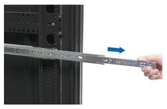
**3** Align the fixing holes of the inner rail to the attachment points on the side of the chassis. Slide the inner rail away from the front panel to attach it to the chassis.
