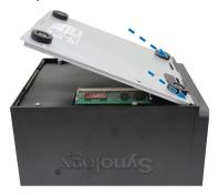
**6** Reconnect the cables you removed in step 1, and then press and hold the power button to turn on your Synology NAS.
