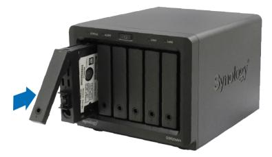
Important: Make sure the drive tray is completely inserted. Otherwise, the drive might not function properly.
