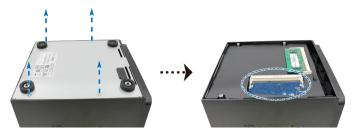
*Important:* When you remove the panel, the sensitive internal components are exposed. Avoid touching anything other than the memory assembly when you remove or add a memory module.
