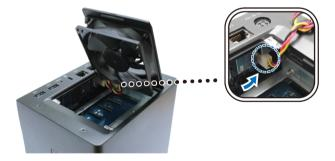
5 Slide one side of the fan into the Synology NAS first then close the fan case.
