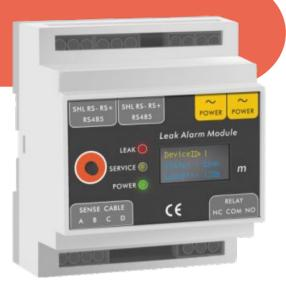
**The SYSG5002 Positioning Detection Module** can detect the leakage of water, acid-base, oil and other liquids, and connect the sensing cable up to 1500 meters. When a liquid leak is detected, the leak location is displayed via the LCD screen and the relay alarm signal is issued
